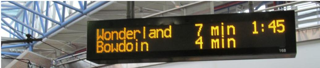
As represented last year, the subway countdown displays predicted arrival times of subway trains on existing LED signs at Red, Orange and Blue Line stations using new in-house prediction software and modified sign software.
